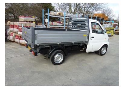
The Tipper is a truly unique vehicle that features a payload of 665kg together with a three way tipper operation. This gives the operator the flexibility of tipping the load bed not only rearwards but also to the left and right. This operation can be controlled both from within and outside of the cabin.
