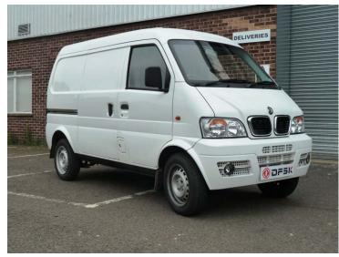
The van offers a payload of 548kg with a load capacity in excess of three cubic metres giving the lowest price to load area and payload of any small LCV. To achieve this the load area features a maximum and minimum width of 1,300 and 1,030 mm together with limited wheel arch intrusion.
