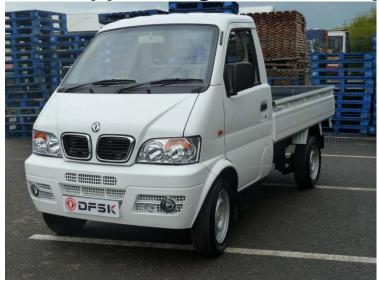
The Single Cab Pickup is a unique vehicle, offering a payload of over 900kg carried within drop down sides and tail gate giving the user easy loading and unloading of the flat load bed.
